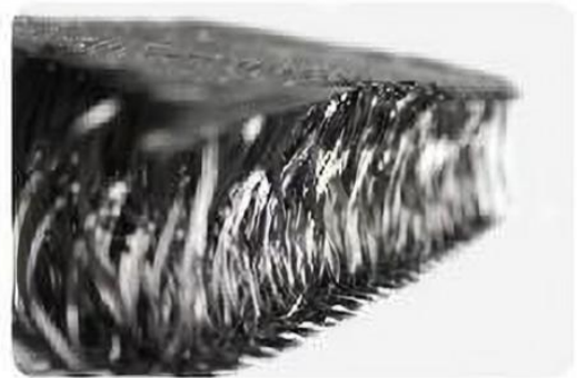
中空层联结构织物 Linking structure with hollow inside.
